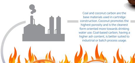
Coal and coconut are individually heated to 870°C in a carbon activation furnace.
